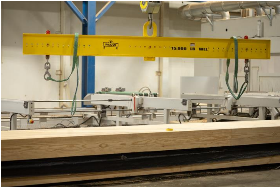
Figure 20: A large Southern Yellow Pine glulam element awaits processing.
